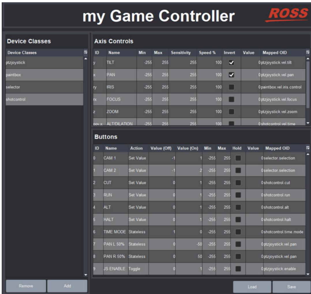
Figure 35 - Mapping USB controller inputs (shown with Device Classes added and controls mapped to OIDs)
