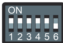
Figure 10 - DIP switches, set for normal operation
