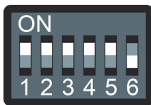
Figure 5 - DIP switches, set for normal operation
