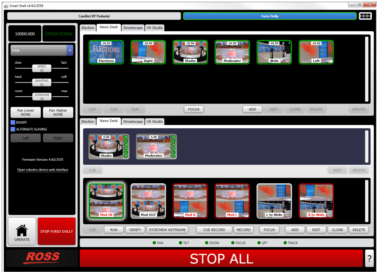
Figure 54 - SmartShell Main Window, showing controls for a Furio Dolly
