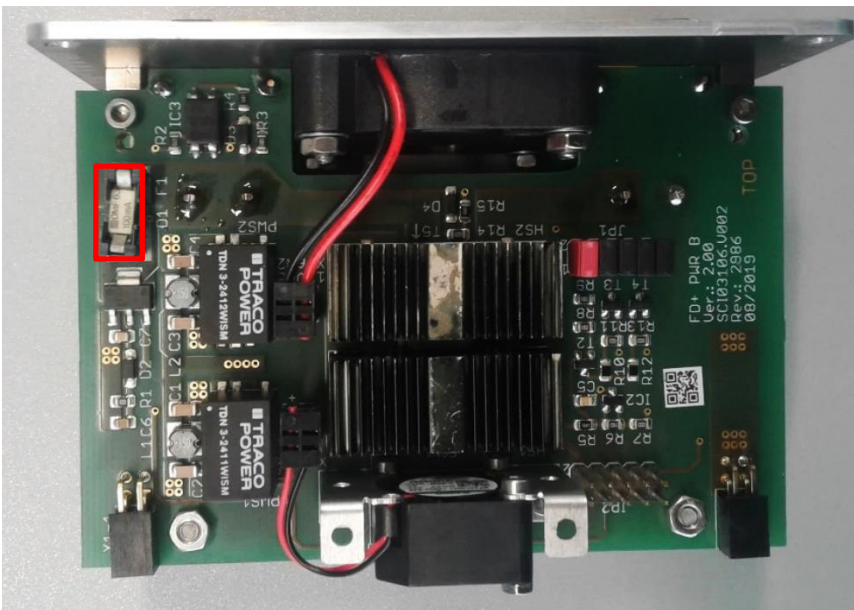
FIGURE 6: FUSE-LOCATION ON THE TOP POWER-BOARD
