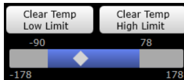
Figure 101 - - Axis Bar and Limit Buttons, with Low (-90) and High (78) Temporary Limits Set
