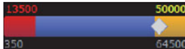
Figure 96 - The Axis Bar for the TRACK Axis, showing a Collision Avoidance Limit (red value and bar) and a Reflector Limit (yellow value and bar). The Reflector Limit is shown only while the dolly is at the limit or is beyond the limit (which can occur if the dolly approaches the reflector at high speed).
