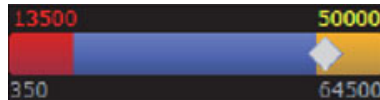
Figure 99 - The Axis Bar for the TRACK Axis, showing a Collision Avoidance Limit (red value and bar) and a Reflector Limit (yellow value and bar). The Reflector Limit is shown only while the dolly is at the limit or is beyond the limit (which can occur if the dolly approaches the reflector at high speed).
