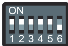
Figure 5 - DIP switches, set for normal operation
