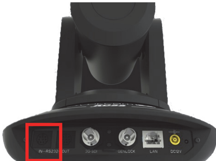
Figure 7 - PIVOTCam-SE (rear view), with red box showing the RS232 IN port
