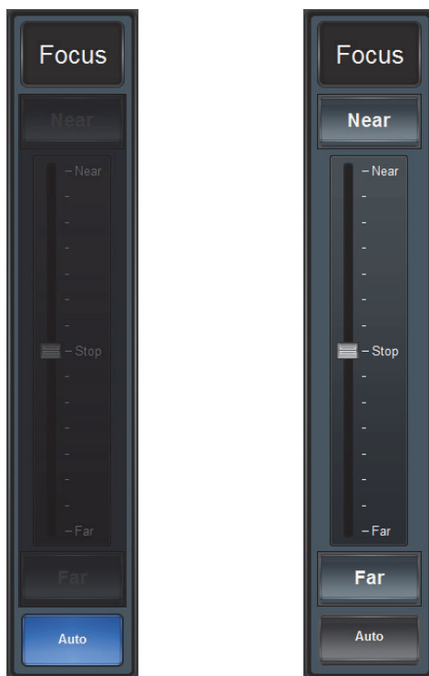
Figure 3.23 - Focus Controls - Auto Focus (left), and Manual Focus (right)
