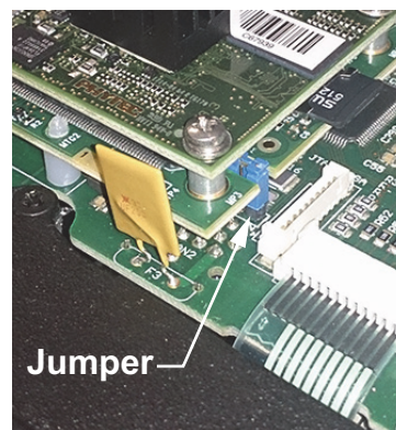
Figure 6 - Blue Jumper on Main Circuit Board, Before New CPU Module Installation (left) and After (right)
