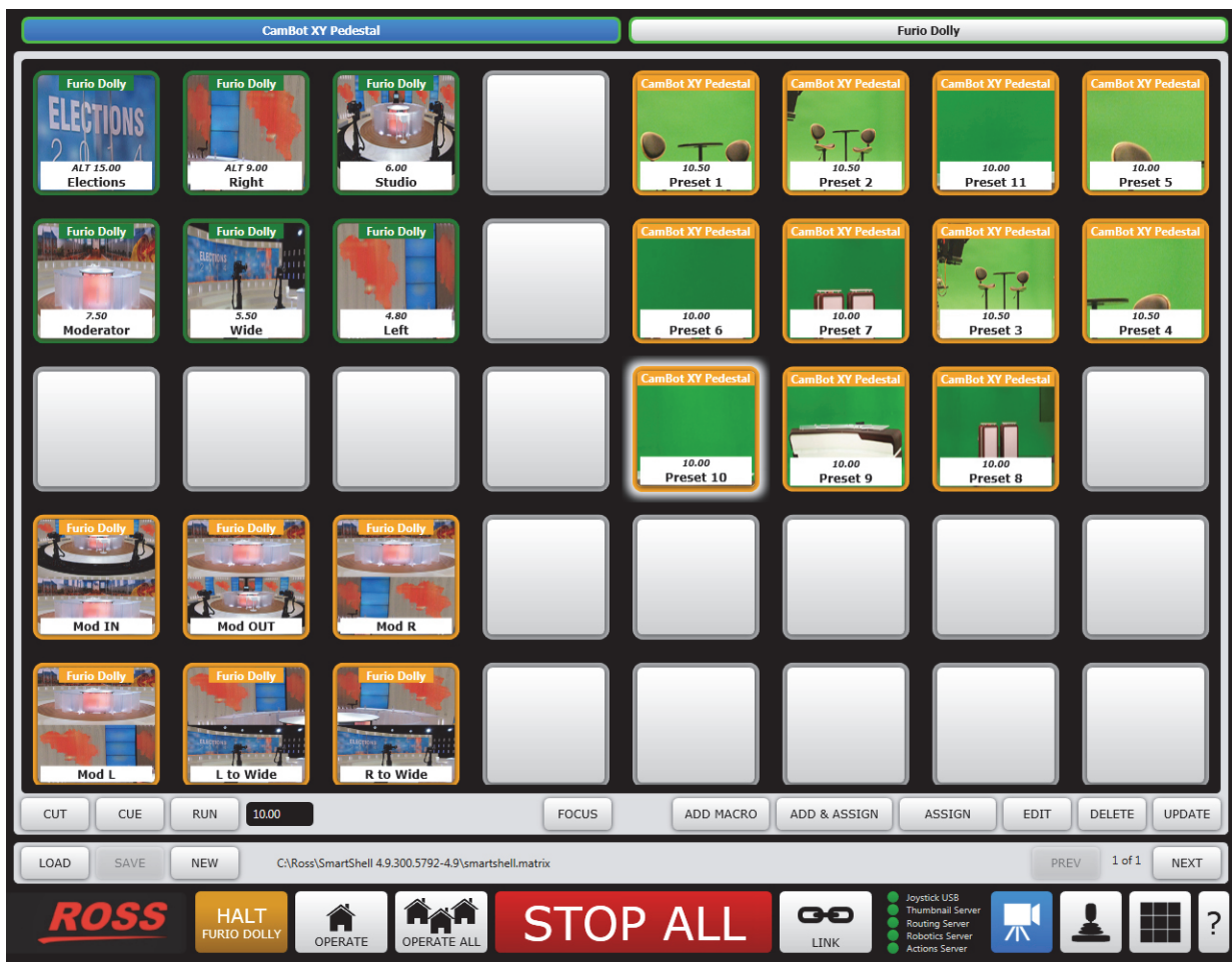
Figure 1 - The SmartShell Control Application (in Matrix View for Panel Mode), Controlling CamBot and Furio Robots
