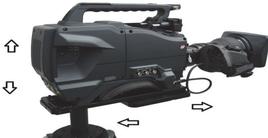
Figure 3.11 - Camera/Lens Properly Balanced
