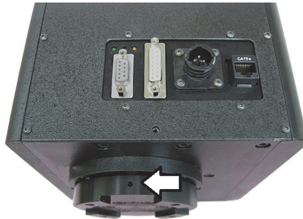
Figure 3.4 - Pan Base in Correct Position
