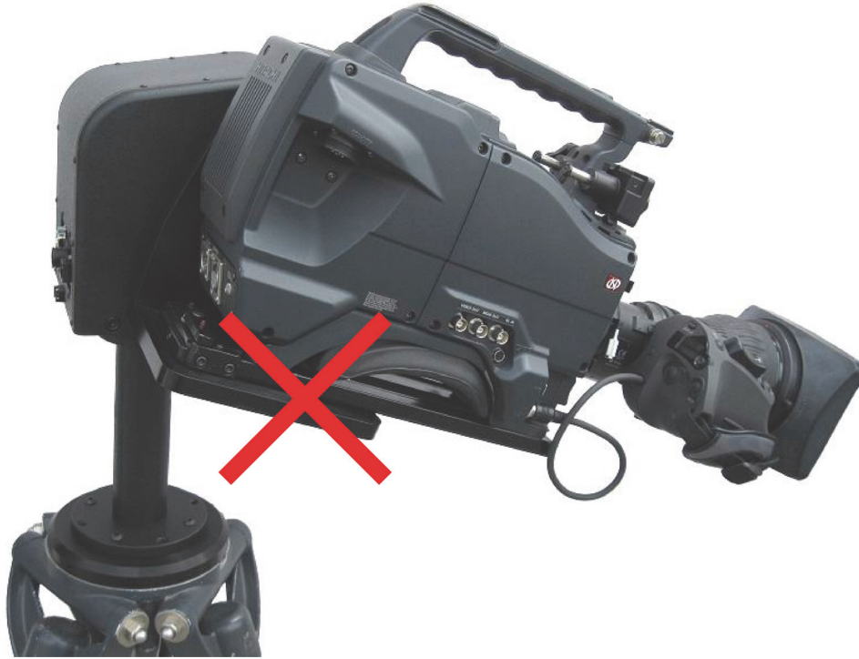
Figure 3.10 - Camera/Lens Mounted but Out of Balance
