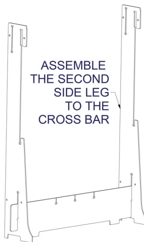
Figure 2 - Attaching the Second Side Leg to Complete the Frame Base
