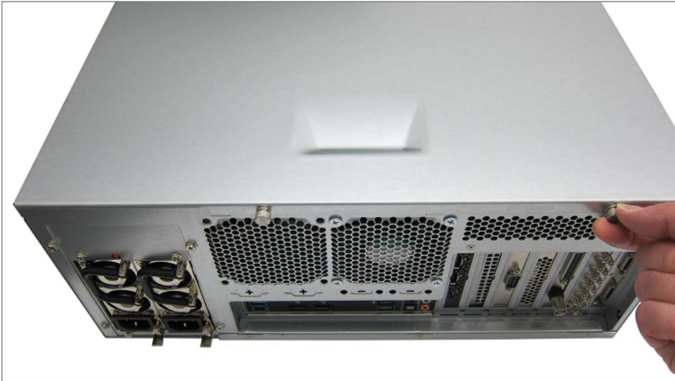
★ Set the two thumbscrews aside, as they will be needed to replace the top panel.
