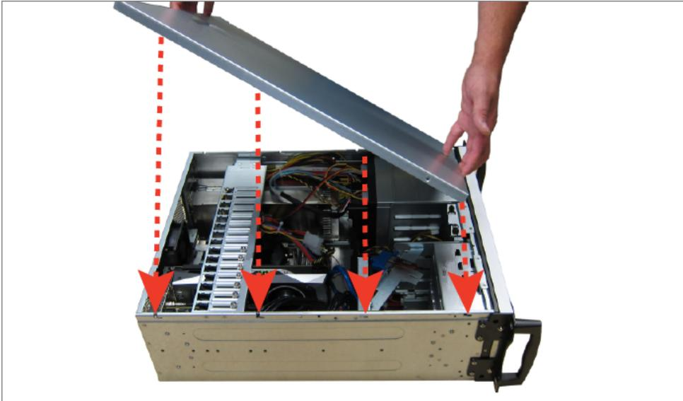
6. Gently slide the top panel into place, until a clicking noise is heard and the top panel is flush to the front top of the XPression system.
