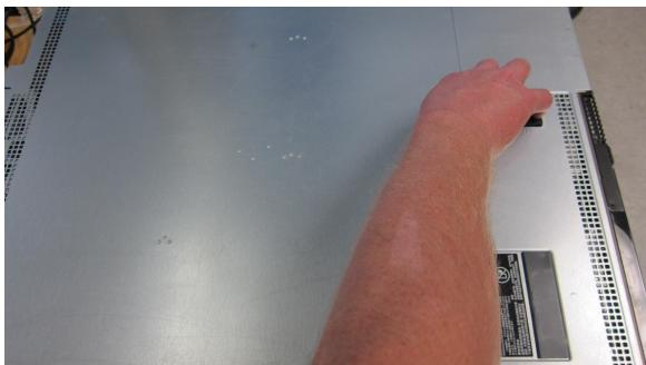
12. Lock the cover lock using a Phillips or flathead screwdriver.
