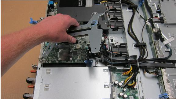
6. Place the card on the riser bracket, lining up the card connectors with the riser bracket connectors.
