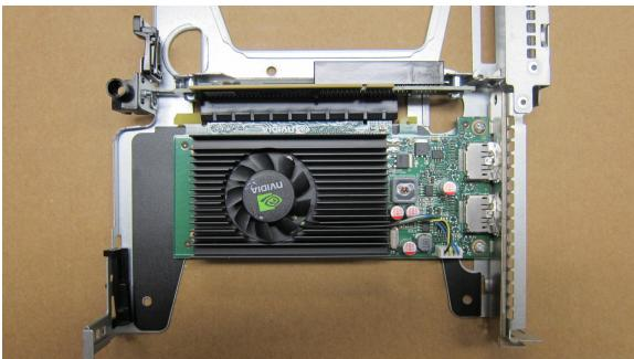
8. Insert and secure the riser bracket to the server.
