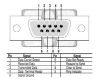
★ To create an RS232 based GPI trigger simply create a device that short-circuits either pin 8-7 or 6-7 on the 9 PIN D-SUB Female connector. It is essential that no additional power is added to the circuit, as that will damage the RS232 port.
