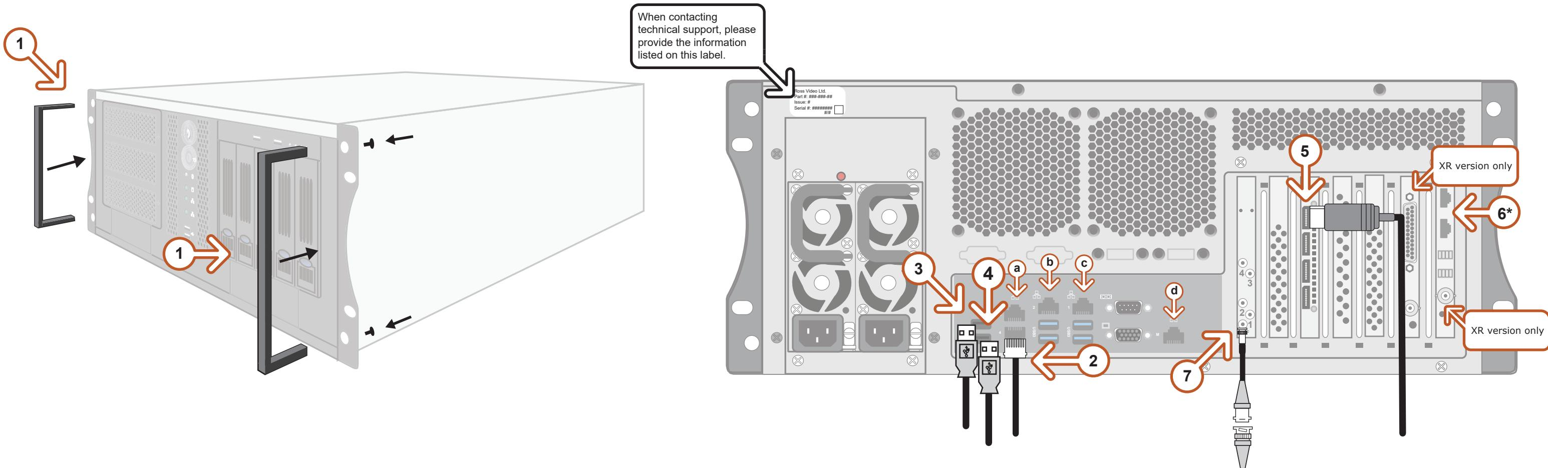
1 Attach the handles to the front rack-mount tabs by aligning the handle with the round holes and fastening from the rear with the supplied screws.
