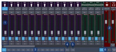
1. **Audio Channel Strips** — Each strip controls the input from that audio channel. Strips are color coded for where the audio comes from. The controls available on each strip
