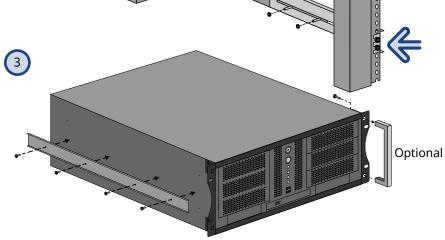
**Note:** Do not use the optional handles to lift the server. The handles are intended to assist with pulling the server from the rack only.
