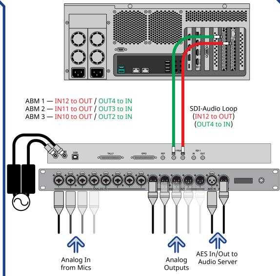
**Important:** Ensure that Phantom Power is turned off for the Analog Input unless you are connecting a microphone that requires phantom power. Connecting the line out from an audio device to the analog input with phantom power on could damage the audio device and/or the 1RU Audio Breakout Module. For added safety, a TRS phone connecter should be used for line in audio sources.
