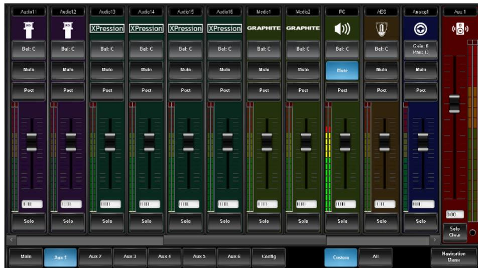
First thing is to set all of the faders to “Post” mode and double click on the “Fader Slider Control” so that it opens to 0 db. This will set the audio to unity gain “AFTER / POST” the Main Mix Faders.
