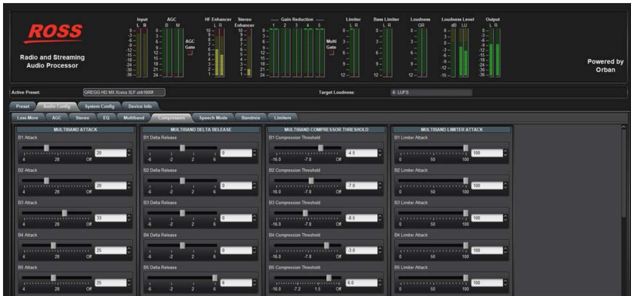
Figure 19.1 Example of the Compressor Controls in Dashboard
