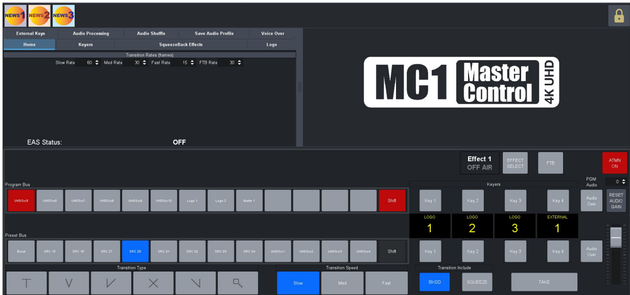
Figure 19 Example of the Channel Select Row of the On Air Control Interface
