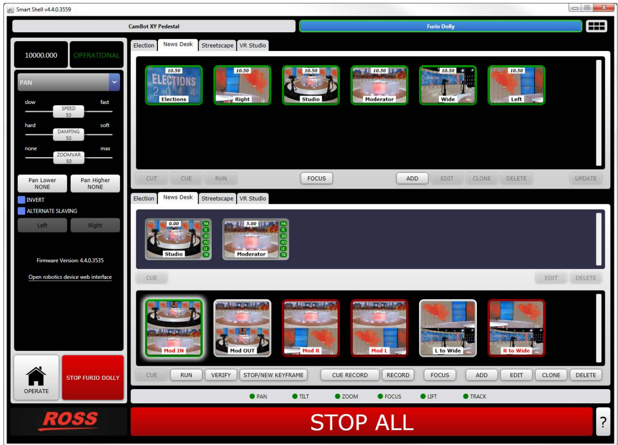
Figure 48 - SmartShell Main Window, showing controls for a Furio Dolly
