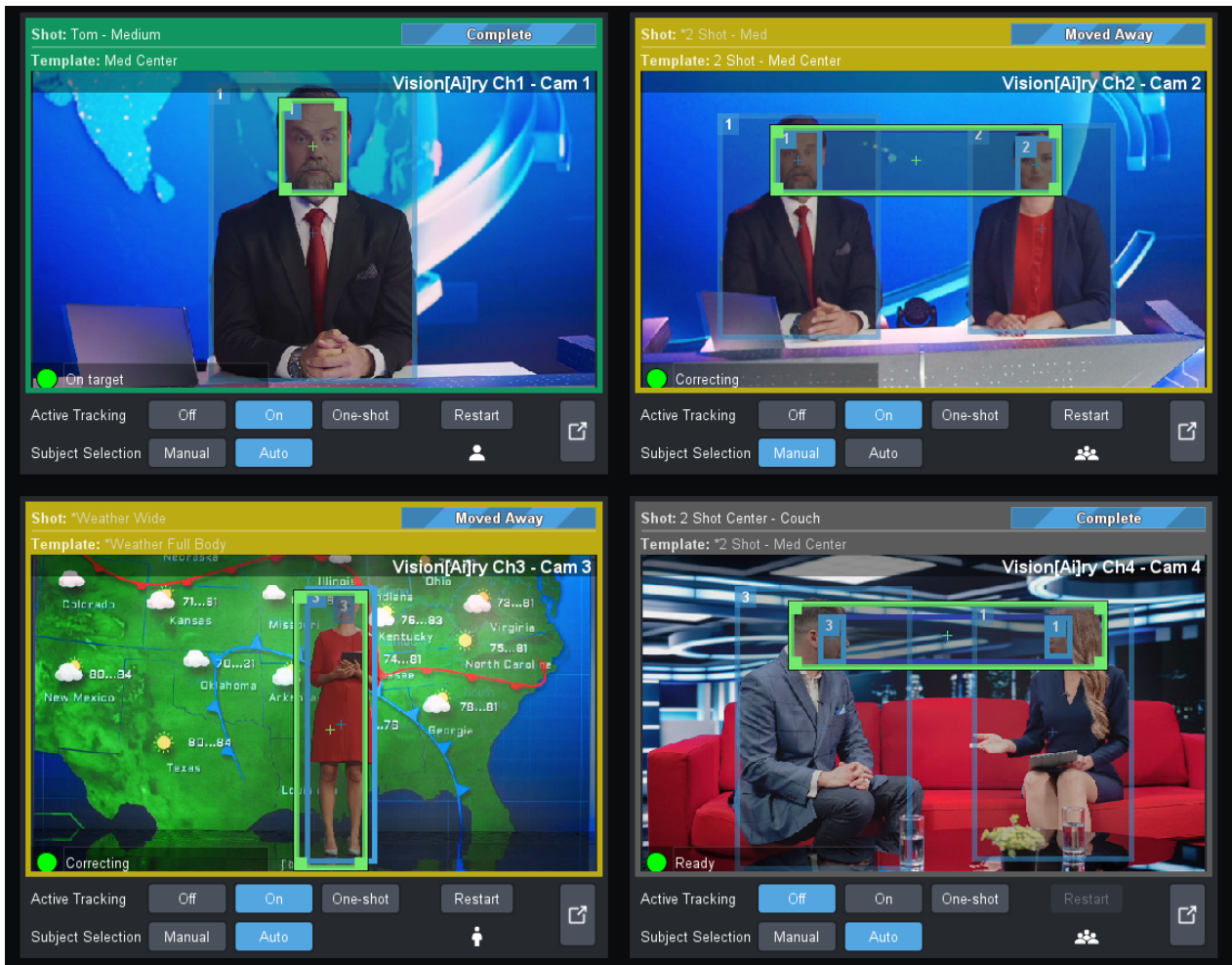
Figure 36 - MultiChannel Page, showing Live Video and Tracking Controls for Four Channels
