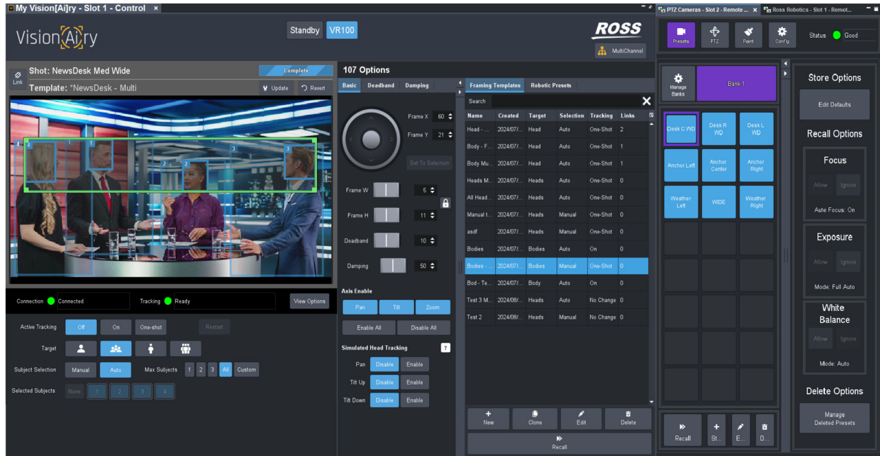
Figure 43 - Example Layout showing Channel Control Page and PT/PTZ Control Pages
