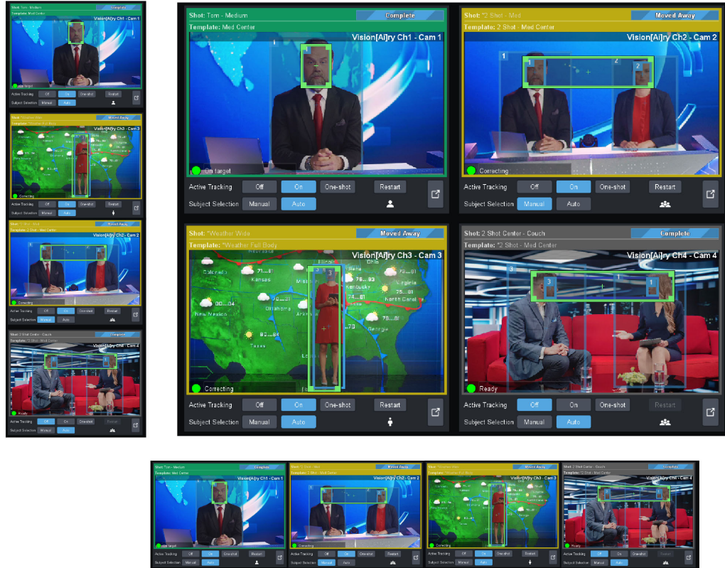
Figure 76 - Four Channel Views Arranged as a Vertical Ribbon (left), as a grid (right), as a Horizontal Ribbon (bottom)
