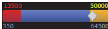
Figure 88 - The Axis Bar for the TRACK Axis, showing a Collision Avoidance Limit (red value and bar) and a Reflector Limit (yellow value and bar). The Reflector Limit is shown only while the dolly is at the limit or is beyond the limit (which can occur if the dolly approaches the reflector at high speed).
