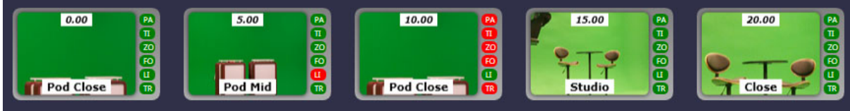
Figure 42 - A Move in which the Start of the Lift Axis is Delayed Until the Third Keyframe
