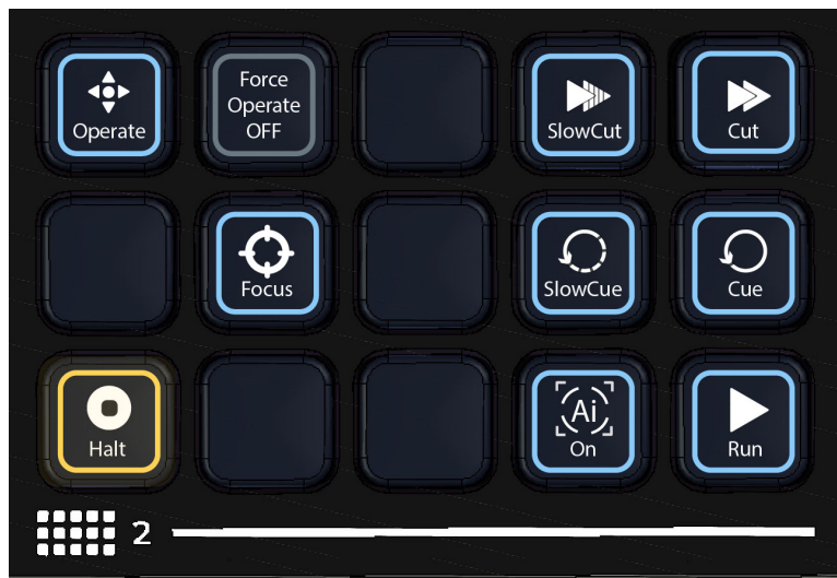
Figure 76 - CX-3R Joystick Panel Camera Selection Buttons (button appearance subject to available functionality)
