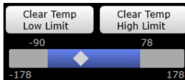
Figure 104 - - Axis Bar and Limit Buttons, with Low (-90) and High (78) Temporary Limits Set
