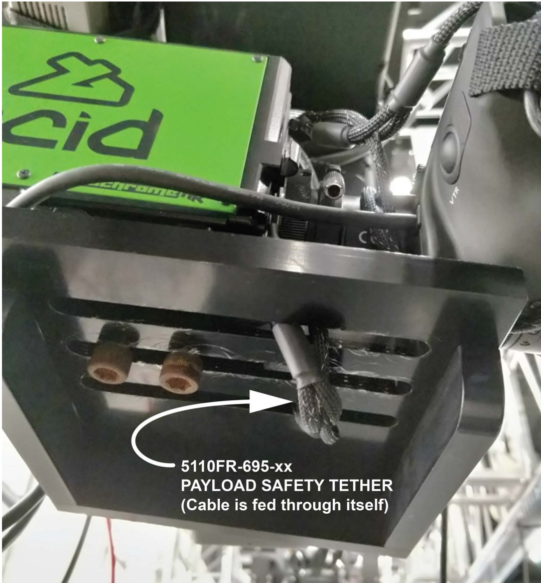
Figure 36 Payload Safety Tether Secures the Camera Cradle
