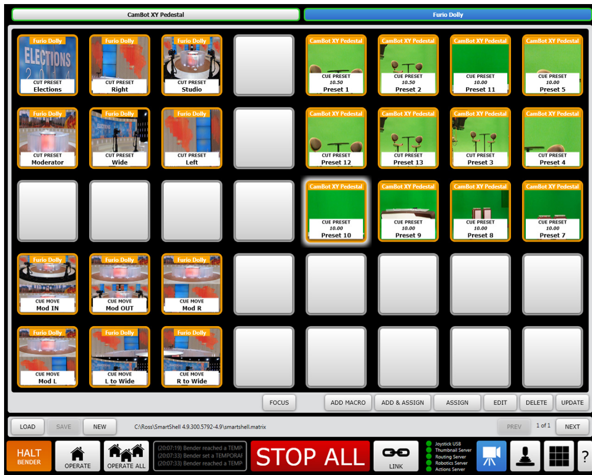
Figure 21 - The SmartShell Control Application (in Matrix Mode), Controlling CamBot and Furio Robots
