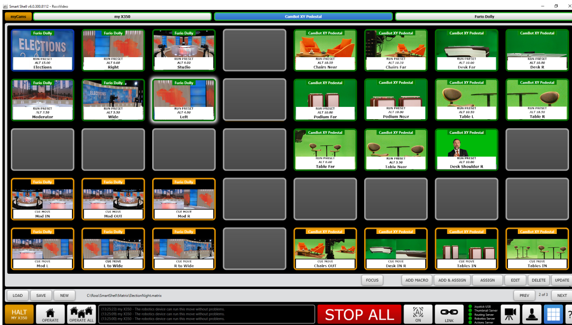
Figure 14 - The SmartShell Control Application (in Matrix Mode), Controlling CamBot and Furio Robots
