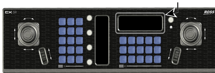
Figure 4.4 CX-3R Joystick Panel Display to Set the IP Address
