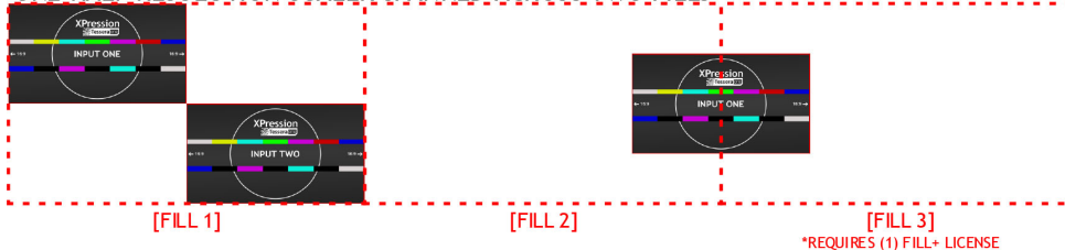
TWO HALF RESOLUTION SCALERS AVAILABLE ON ONE FILL ONE HALF RESOLUTION SCALER SPANNED ACROSS TWO FILLS
