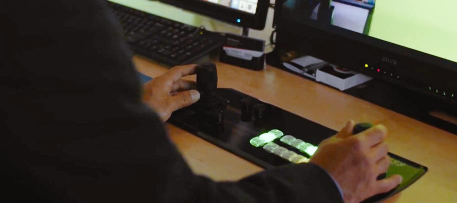
Each SmartShell control station communicates with the robots over an Ethernet infrastructure using an open API, simplifying integration into new or existing
